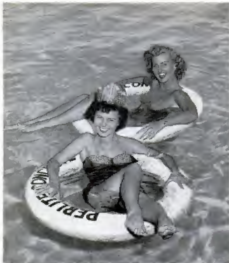
Life preservers made from solid perlite concrete float easily. Weight of perlite concrete is 25 to 35 pounds per cubic foot
